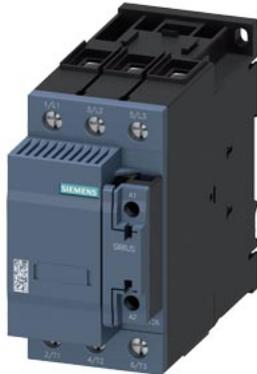
Kondensatorschütz, AC-6b 50 kVA<sub>r</sub>, / 400 V 1 S + 1 Ö, AC 220 V, 50/60 Hz
