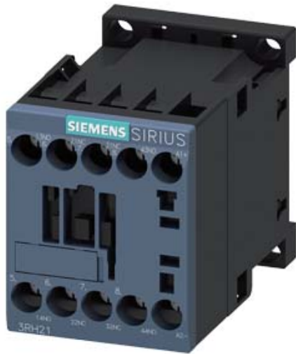
CONTACTOR RELAY, 2NO+2NC, DC 24V, SIZE S00, SCREW TERMINAL
