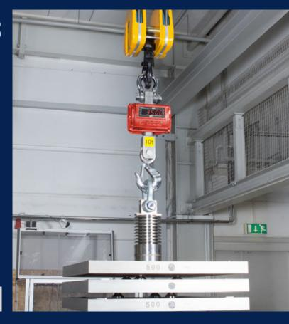
Do you use your crane scales in ISO-certified processes or where verification is mandatory? Then we can produce the right calibration certificate or the relevant Declaration of Conformity for your measuring device. Thanks to a modern crane scale test unit, we can calibrate or verify crane scales and force-measuring devices from any manufacturer to a maximum load of up to 12 t or 120 kN.
