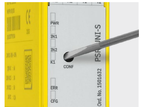
Confirmation of the configuration settings directly on the device
